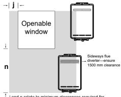
$^{\dagger}\,$  j and n relate to minimum clearances required for balanced flue terminals from AS/NZS 5601.1
