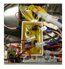
The Rinnai INFINITY error indication switch is a volt-free, normally open switch. The switch will shift to a closed position when there is an active error in the water heater.
