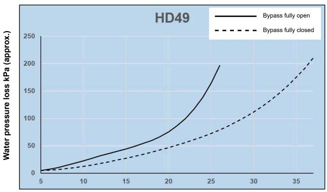
Water flow rate L/min
